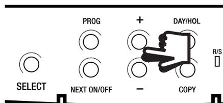
3. Press the **PROG** button to return the unit to **RUN** mode (time appears and the colon in the display begins to flash).
