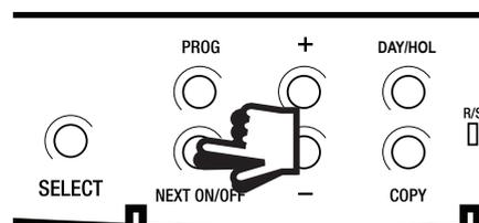
4. Continue programming the system **ON** and **OFF** times in this way by using the + or - buttons to set the time you want and pressing the **NEXT ON/OFF** button to move to the next setting.
