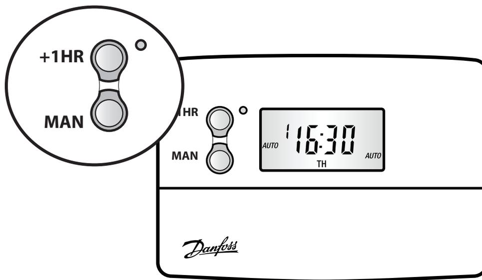
**+1HR** Pressing this button when the unit is in **AUTO** or **ALLDAY** mode will cause the system to remain on for an extra hour. If it is pressed while the programme is **OFF** the system will come on immediately for 1 hour then go off again. **+1HR** will be shown in the display.
