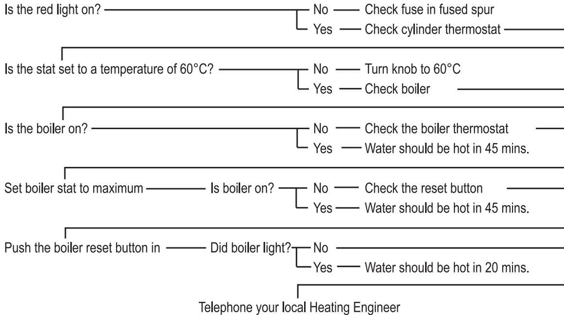
After the water has been heated, return the programmer and other controls to the required settings.
